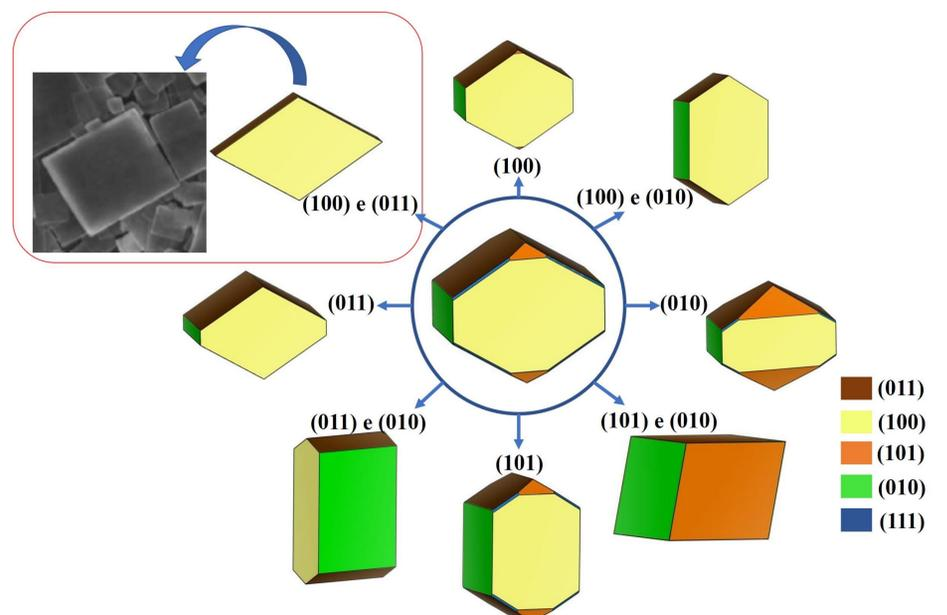
Figure 3: Morphology map of  $\beta$ - $\text{Li}_3\text{PS}_4$ . In the center, is the ideal crystal. Each arrow indicates the direction of stabilization of one or two surfaces by decreasing the  $E_{surf}$ . On the left, is the SEM of  $\beta$ - $\text{Li}_3\text{PS}_4$  obtained by Hood and co-authors[2].
