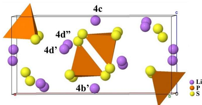
Figure 1: Optimized Pnma structure of  $\text{Li}_3\text{PS}_4$  with Li Wyckoff positions (4b', 4c, 4d', and 4d'').
