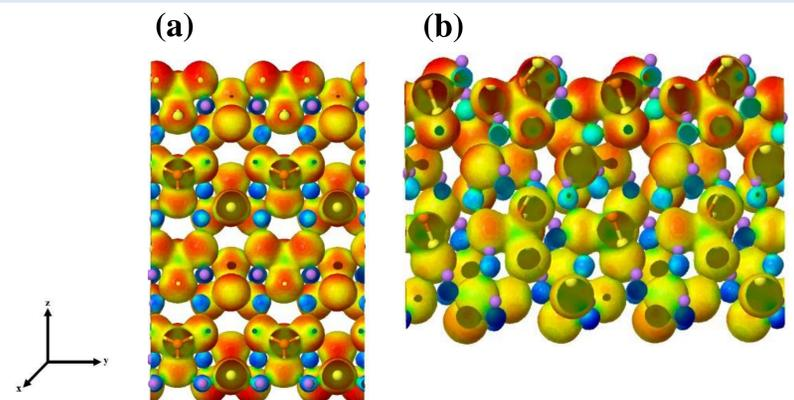
Figure 2: Three-dimensional maps of the electronic charge density superimposed to the electrostatic potential of  $\beta$ - $\text{Li}_3\text{PS}_4$  surfaces along z-direction: (a) (100) and (c) (011). The scale maps range from negative (-) in blue to positive (+) in red.
